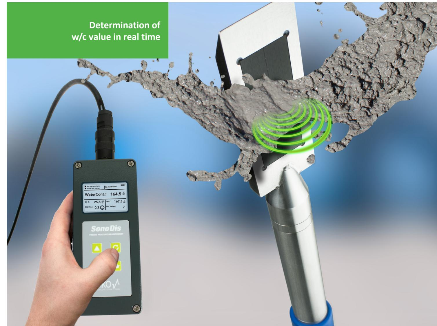
Based on the revolutionary TRIME radar technology, it is possible for the first time to determine the water content of fresh concrete quickly, precisely and directly on site.
