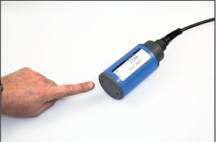
A hand is shown pressing one of the black O-rings into one of the holes on the bottom of the blue sensor body. |
