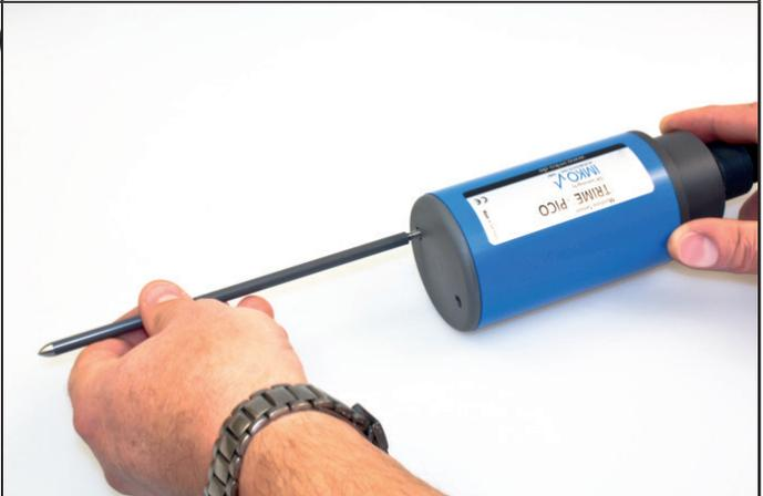
A hand is shown screwing one of the black probe rods into the hole on the bottom of the blue sensor body.     |
