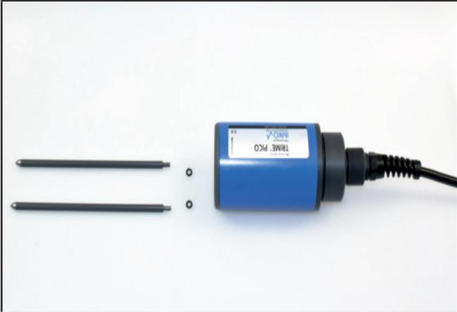
A blue cylindrical sensor body with a black cable is shown next to two black probe rods and two small black O-rings. The sensor body has a label that reads 'TRIME PICO' and 'IMCO'. |
